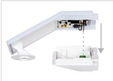
Fig. 15 Push the lid on the lower part. This also makes the plug-in connection between the board in the lid and the socket in the lower part.
