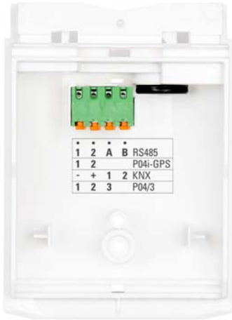
Fig. 14 Connect KNX data (+/-) and power supply (12...40V DC, 12...28V AC, 1|2) to the connector.
