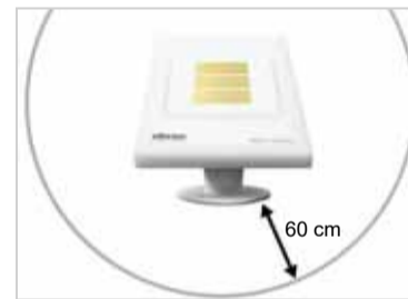
Fig. 1 There must be at least 60 cm clearance to other elements (structures, construction parts, etc.) below, to the sides and in front of the device.
