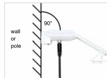
Fig. 2 The device must be attached to a vertical wall (or a pole).
