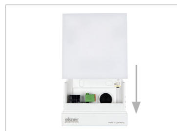
Fig. 13 Put the cover on the lower part. This also makes the plug-in connection between the board in the cover and the socket in the lower part.
