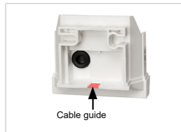
b) If the power lead is to be surface-mounted, the cable guide is broken off. The lead is then fed into the device from the bottom of the housing.
