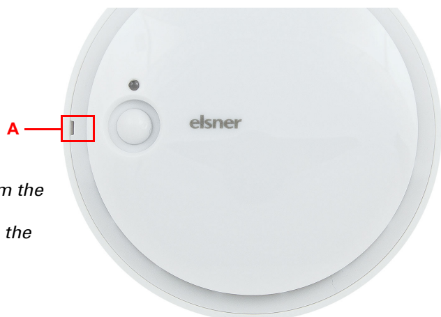
Fig. 3 Open the housing. To do this, carefully lift the cover from the skirting. Start at the recess, e.g. with a flat-head screwdriver.
