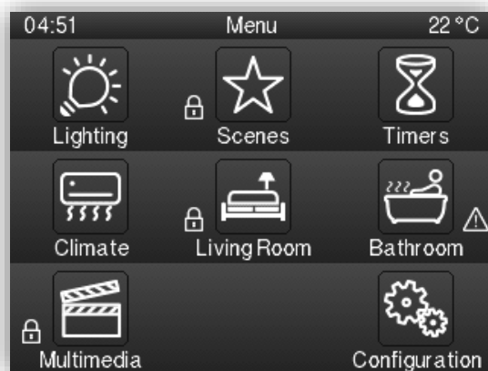
Figure 24. Menu with protection and alarms.
