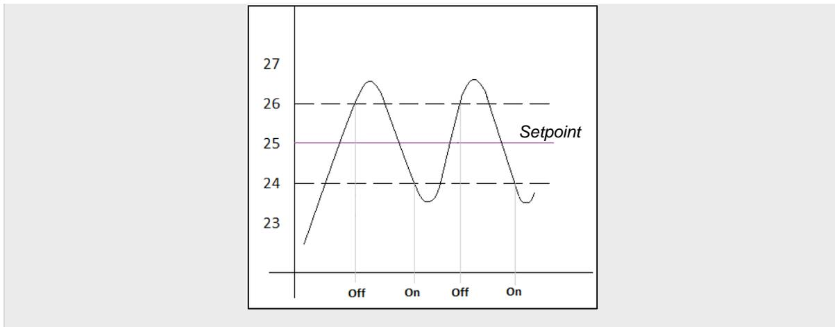
The main disadvantage of this algorithm, when compared to other advanced systems, is the permanent fluctuation around the setpoint temperature, which has a direct impact on the power consumption and on the comfort:
