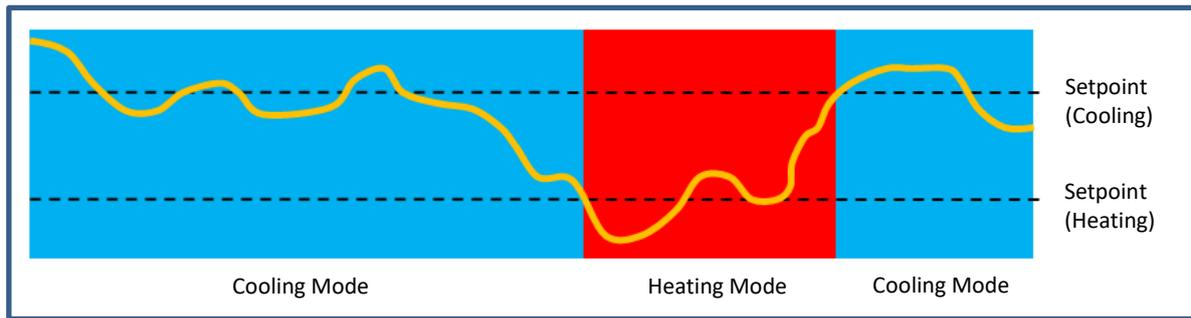
Figure 1. Automatic Mode Switch.
