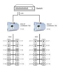
KNX IP LineMaster 762 as line coupler
