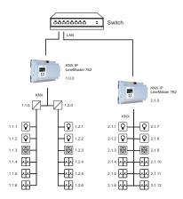
KNX IP LineMaster 762 as area and line coupler
