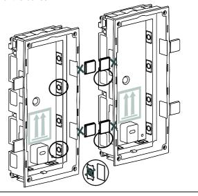
Assemble the boxes by using the auxiliary parts (A and B) and the tube-shape parts. Fix it with the screws.
