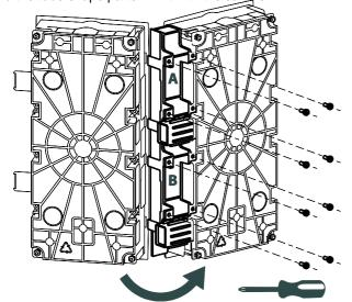
Place the assembled box in the hole, recover the cables and fix the flush-mount box to the drywall by means of the screws that adjust the flaps to the drywall thickness. Please, pay attention to the top orientation mark.
