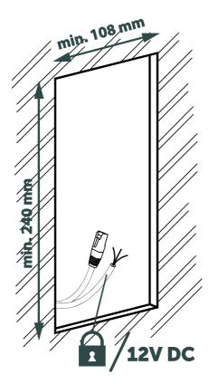
Place the box in the hole, recover the cables and fix the flush-mount box to the drywall by means of the screws that adjust the flaps to the drywall thickness. Please, pay attention to the top orientation mark.
