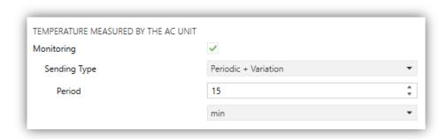
Figure 6 AC Gateway. Configuration. Temperature measured by the AC unit.
