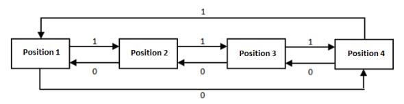
Figure 13: Cyclical flap step control (4 positions and no swing function)
