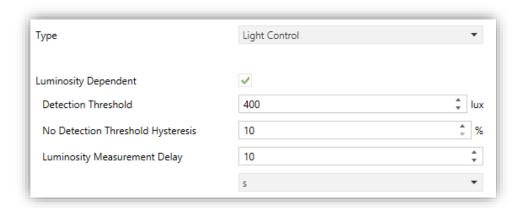
Figure 6. Light control channel
