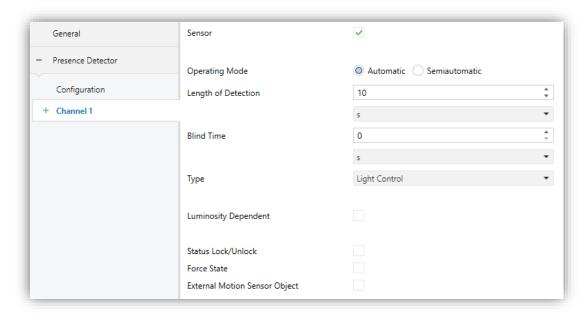
Figure 5. Presence detection – Channel i
