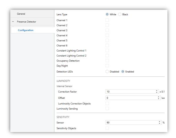
Figure 1. Presence detector - Configuration
